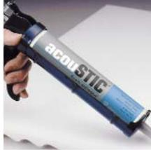
acouSTIC adhesive (part number PA-02) is a nontoxic, water-based adhesive that cleans up with soap and water. Each 10.5-ounce tube installs approximately 32 square feet of product. Tubes fit standard caulking guns or can be used with pinta's applicator gun.
