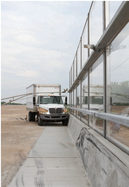
A 22,180LBS (10,060KG) TRUCK IMPACTS THE MASH TL-4 SYSTEM AT 58MPH ON A 15°ANGLE
