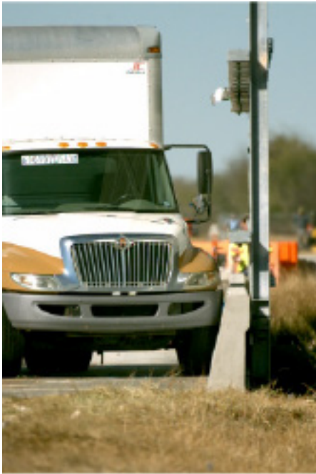
A 22,500 LBS (10,206 KG) TRUCK IMPACTS THE MASH TL-4 SYSTEM AT 58MPH ON A 15° ANGLE
