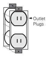
3. Pull the Outlet Plugs away from the wall equal to the thickness of the wall panel.
