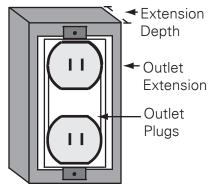
Install Outlet Extension per wall outlet instructions. The Extension Depth is equal to the thickness of the wall panel.
