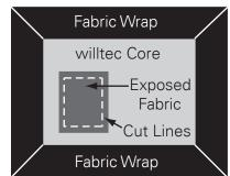
9. Cut a hole in the Exposed Fabric smaller than the whole in the willtec Core.
