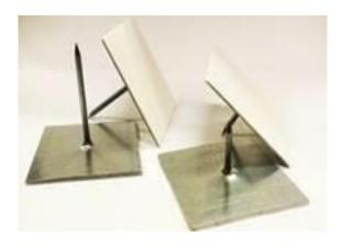
Impaling Pins are steel spindles with corrosion resistant coating. The base plate is 2" square and is made of galvanized steel with a pre-applied, pressure sensitive adhesive (PSA) protected by a release paper. Standard lengths are 3/4" and 15/8".
