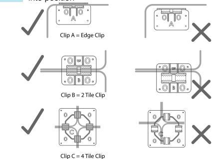
The clips supplies are appropriate for the installation of 9 tiles arranged in a 3 x 3 square pattern.
