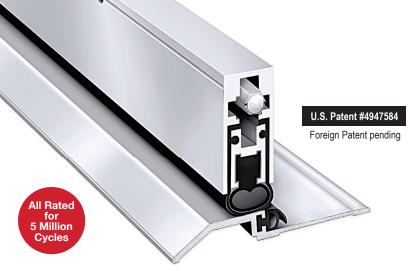
ZERO's patented **automatic door bottom** technology ensures a tight seal against the floor or saddle. As the door is closed, an adjustable "plunger" is compressed against the door frame, activating a concealed flat spring mechanism. This mechanism drops the seal smoothly from the housing in a scissor-like motion as illustrated below. The door seal compresses tightly even on uneven surfaces and retracts automatically when the door is opened.
